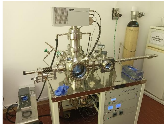
Temperature Programmed Desorption Workstation TPD Workstation – Analysis of Thermal Desorption Products By UHV TPD/TDS
